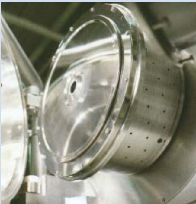
Figure 3a: A horizontal inverting bag centrifuge in 'invert closed' mode. (Image courtesy of Heinkel AG)
