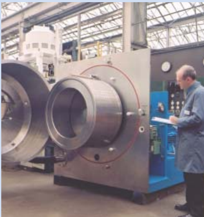
Figure 5: Examples of the horizontal 'through the wall' design that enable the clean and dirty ends of the centrifuge to be kept completely separate. (Images courtesy of Thomas Broadbent & Sons Ltd and Comi Condor)
