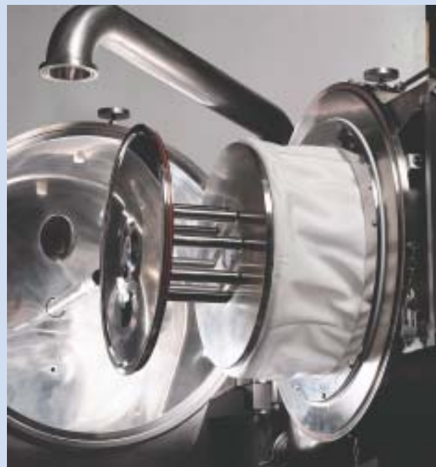
Figure 3b: Horizontal inverting bag centrifuge in 'invert open' mode. (Image courtesy of Heinkel AG)
