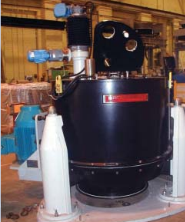
Figure 2: Broadbent 46A centrifuge features an energy-efficient electric drive system. (Image courtesy of Thomas Broadbent & Sons Ltd).
