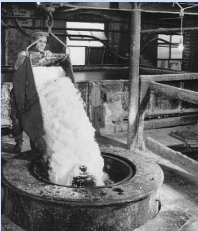
Figure 1: The safe operation of steam driven basket centrifuge installations relied heavily on the operator. (Image courtesy of Thomas Broadbent & Sons Ltd).
