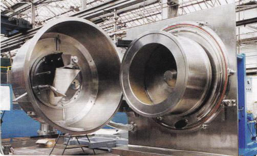
the centrifuge is to be used within the pharmaceutical or fine chemical industry, it may have to be manufactured to a GMP design with an integral CIP system.
