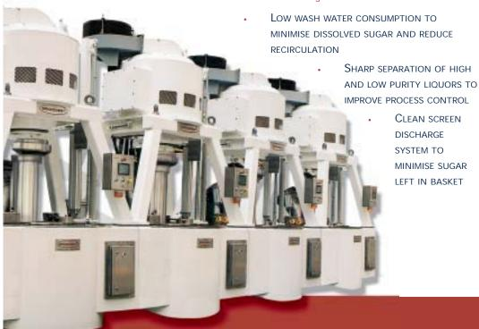
The combination of all these factors make Broadbent batch centrifugals the ideal process solution for the lowest centrifugal operating and maintenance costs
